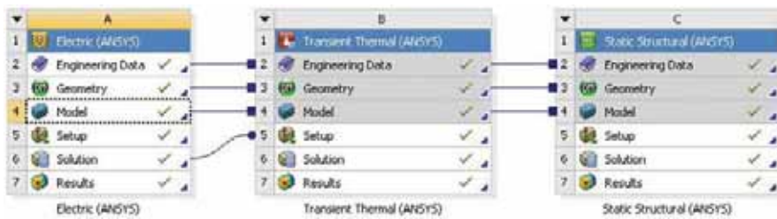
Figure 2 – state flow of the multiphysics analysis
