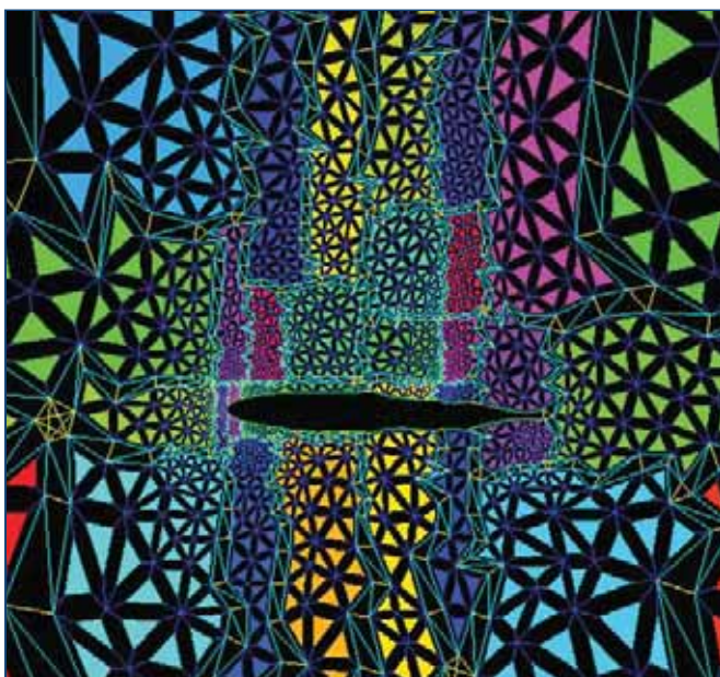
Figure 1 - Computational grid for computing airflow over a wing. Flow is left to the right, the wing is 1.4 degrees from horizontal. The grid is adaptive in two ways: the size of the triangles controls the spatial resolution of the simulation, and the grid is also split into pieces for parallel execution by 32 processors, so that each gets the same number of triangles. Refinement is based on the gradient of the pressure, especially at the leading edge (left) and at the shock. The shock is above the airfoil, 2/3 back. However, there is no shock below the wing: thus the aerodynamics is visible through its effect on the adaptive grid.
