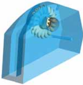
Fig. 3 - Turbine geometry with simplified statoric frame
