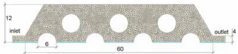
Fig. 9 - The heat exchanger considered in this work. The symmetry axis is highlighted in blue and some dimensioning (in [cm]) is reported.
