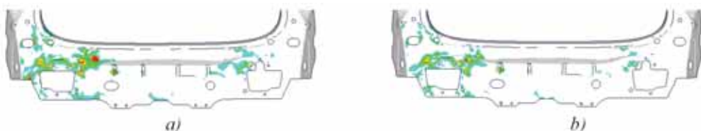
Figure 11: a) shows the plastic strain on the ring frame in the full car model with original bumper beam. b) shows the plastic strain on the ring frame in the full car model with optimized bumper beam.
