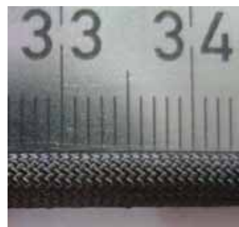
Carbon fiber pipe production test using braiding technology, before impregnation with resin
