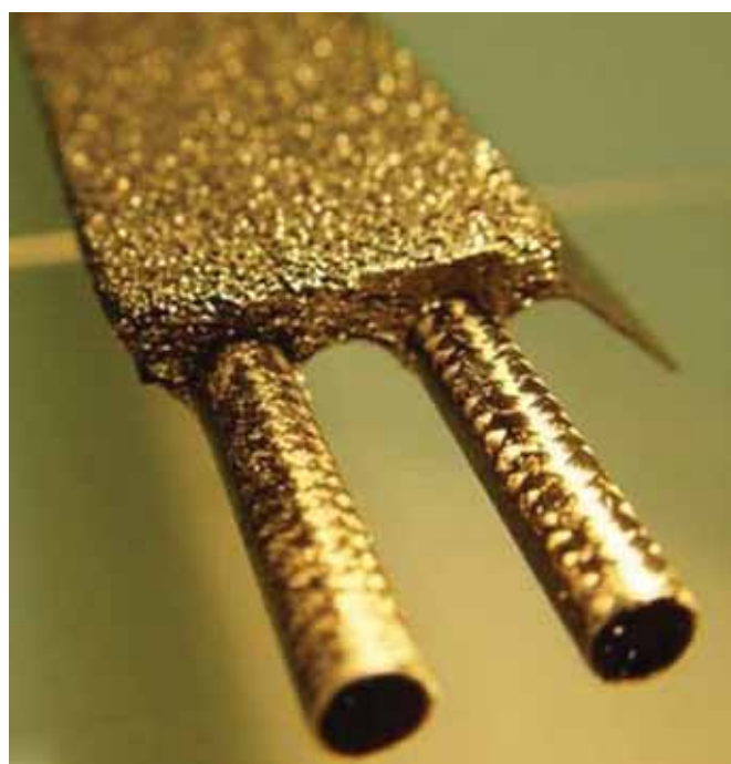
Prototype of a stave with 2 carbon fiber pipes integrated into the carbon foam and attached to the structural omega shaped laminate.
