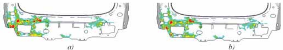
Figure 10: a) shows the plastic strain on the ring frame (i.e. a rear part of car body) in the submodel with original bumper beam. b) shows the plastic strain on the ring frame in the submodel with optimized bumper beam.
