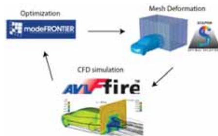
Fig. 3 - A sketch of a single step of the optimization loop, as managed by modeFRONTIER
