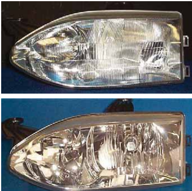
Figure 1: comparison of an old-fashioned glass headlamp (left) and a new transparent plastic headlamp (right)
