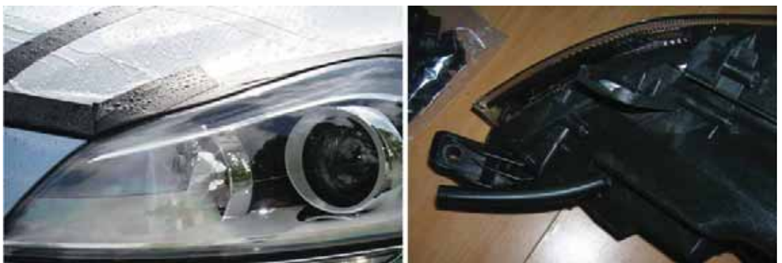
Figure 2: condensate on a prototype specifically designed for enhancing condensate formation. Left: prototype mounted on the car. Right: details of the prototype
