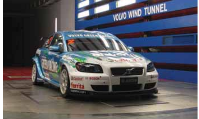
Figure 2: Polestar C30 OGR in the moving-ground Volvo wind tunnel
