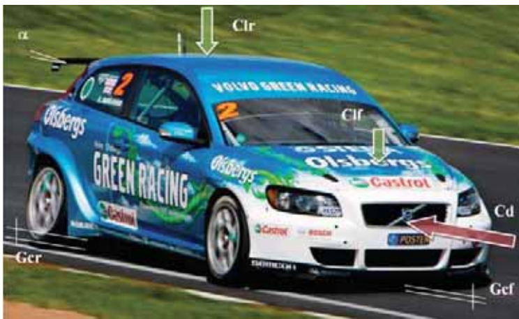
Figure 4: Aerodynamic set-up parameters (inputs) and aerodynamic forces (outputs) on the C30
