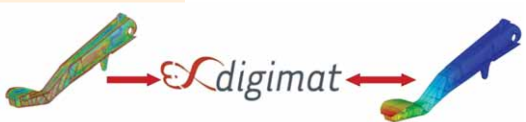
Figure 1: (left) Fiber orientation distribution (from injection molding); (right) Nonlinear structural ANSYS FEA of the pedal where the nonlinear and anisotropic behavior of the material is described by DIGIMAT, taking into account the local fiber orientation.. Models courtesy of Rhodia & Trelleborg.
