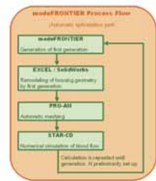
Figure 3. Scheme of the Process Integration realized by modeFRONTIER
