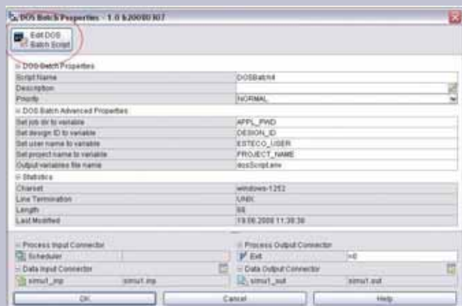
Figure 7: DOS-Batch Properties window in modeFRONTIER v4
