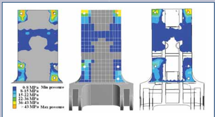
Figure 2: (a) Contact pressure (compressive stress) on the carry-mould as derived by the 3D FE model; (b) pressure applied to the single-body model; (c) resulting compressive stress on the equivalent single-body model.
