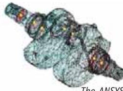
The ANSYS model generated by ANSYS WORKBENCH to obtain the Modal Neutral File
