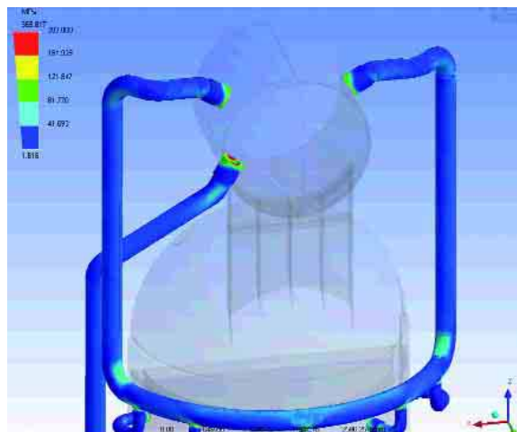
Thermo-mechanical stress analysis on the tubesheet of a S&T heat exchanger
