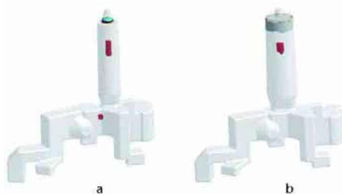
Feeder optimization for the prevention of porosities. (a) initial situation (b) optimized result.
