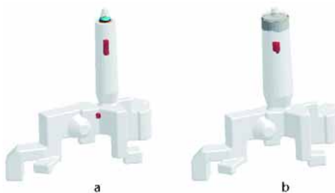
Autonomous feeder optimization for the prevention of porosities. (a) initial situation (b) optimized result.
